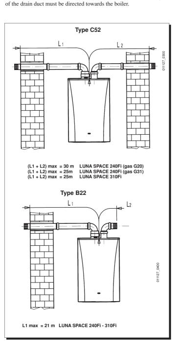
NB: For C52 types, terminals for combustion air suction and combustion product extraction must never be fitted on opposite walls of the building.
