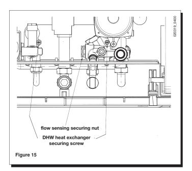
For cleaning the interchange and/ or the domestic hot water circuit we recommend the use of Cillit FFW-AL or Benckiser HF-AL.
