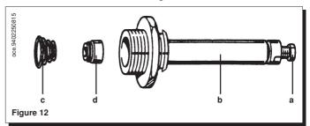
D2) Adjustment to reduced heat output (for HONEYWELL gas valve)
