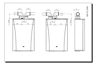
In the case of installation outside the building, or opportunely aired room, it is possible not to connect the suction duct (type B22).
